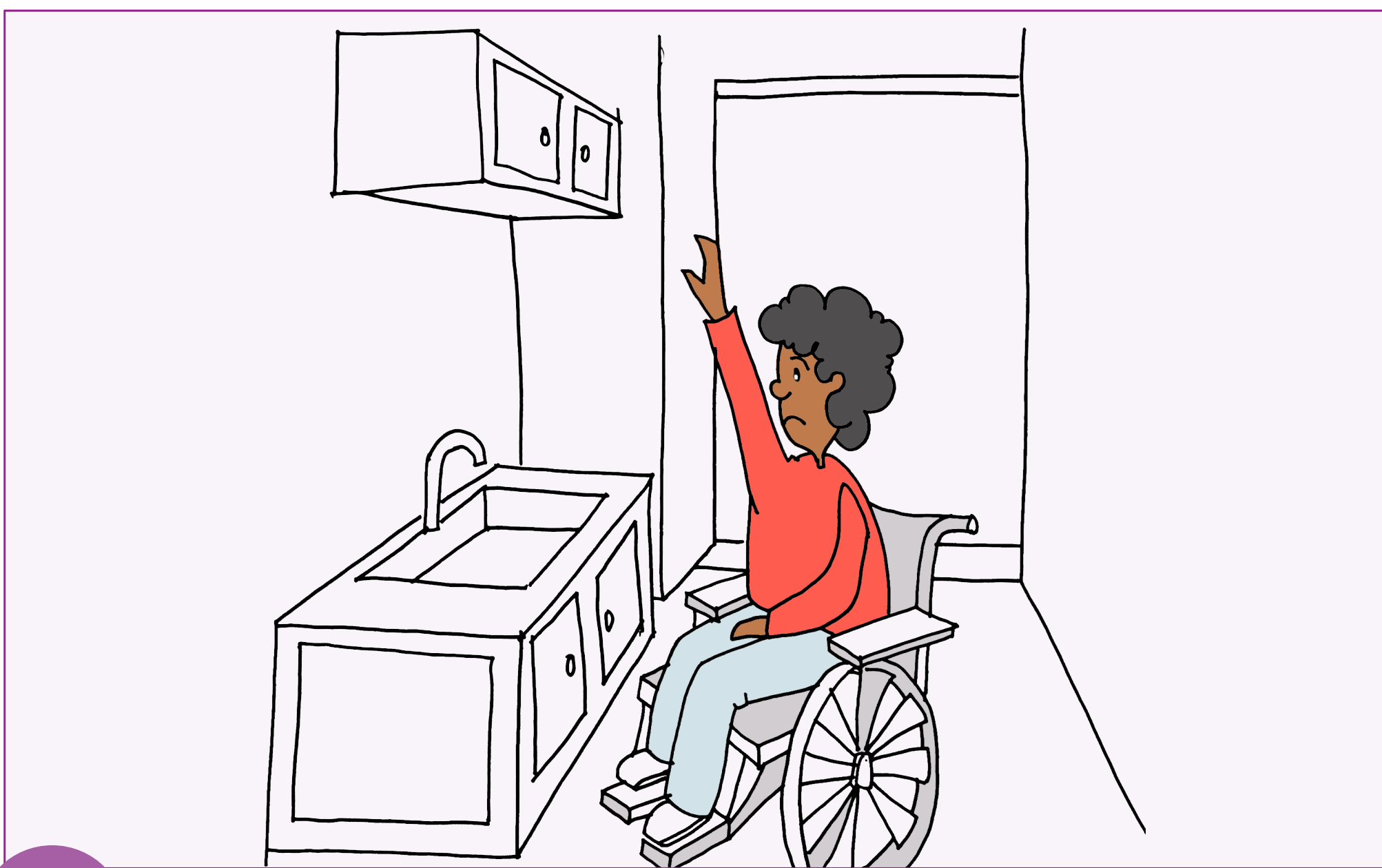
1 Maurine participates in a Universal Design Lab that works with an interior design company to test kitchen design that will be used in a large-scale senior residence project. In the study, she finds the overhead cabinet is too high for people using wheelchairs.
